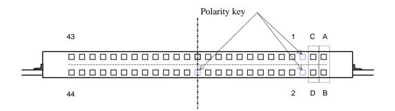
Figure 7 Optional jumper for Drive0/Drive1
